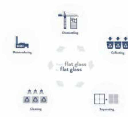
Figure 2 – Closed-loop recycling process for flat glass
