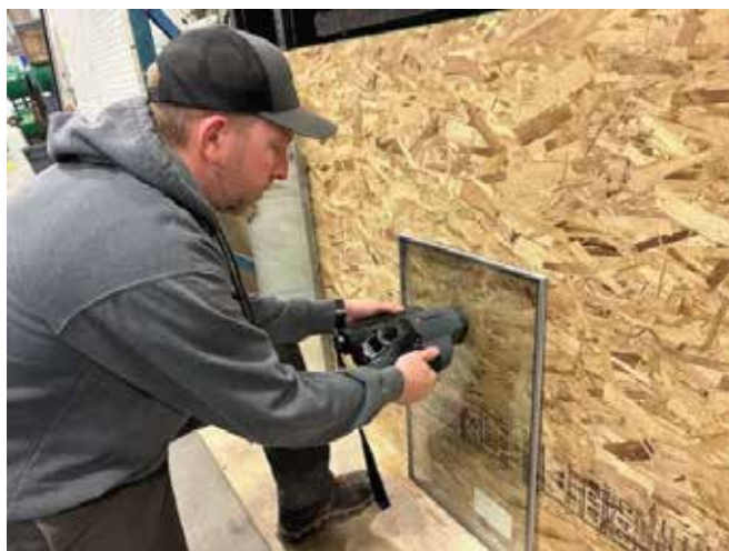
Insul-Lite Manufacturing testing IGUs with Sparklike Handheld™
